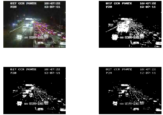
Figure 5: Different Threshold levels (a) Original Image, (b) Threshold Level(0.5), (c) Threshold Level (0.7), (d) Threshold Level (0.8)
